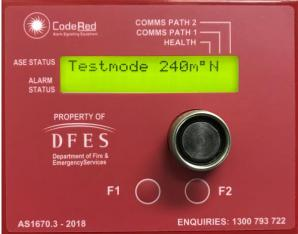
The ASE will automatically exit Test Mode 4 hours after entering Test mode, unless manually returned to normal mode 'AS1670.3-2018'
